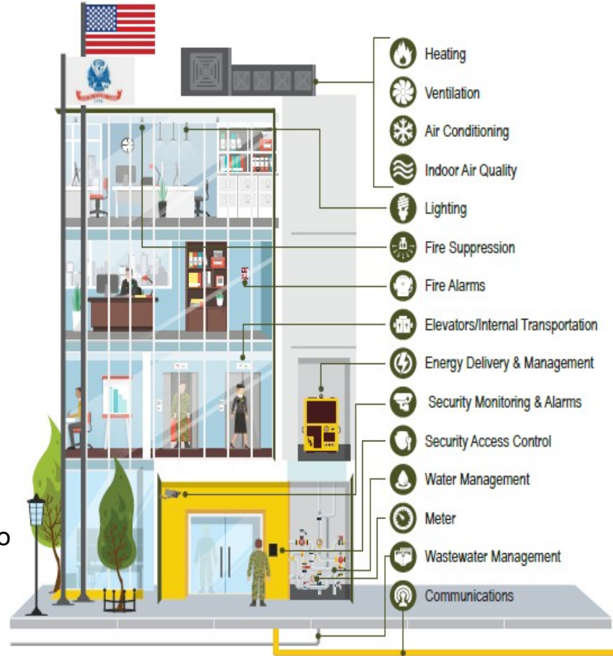
Figure 1. Illustration of the Various Types of Facility-Related Control System
